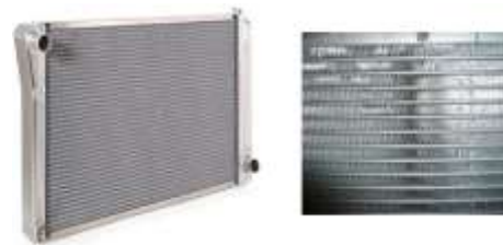
Figure 1 (a) Radiator; 1(b) Radiator with damaged fins
